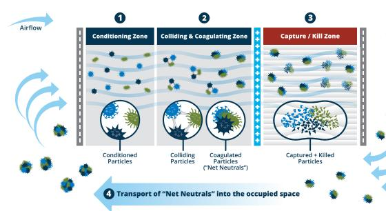
ACTIVE Particle Control Technology conditions particles and pathogens, induces collisions leading to particle coagulation, and then once collected on the capture media kills all biologic matter.
